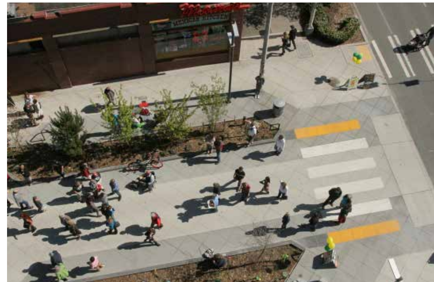
Planting areas provide water quality management and separate pedestrians from vehicles
