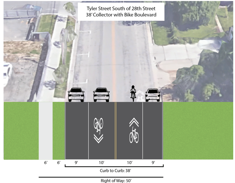
Conceptual cross-section of Tyler Avenue with proposed traffic calming and bicycle facilities
